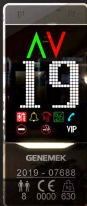
MEGA7V.DM LED 24x16 dotmatrix indicator
