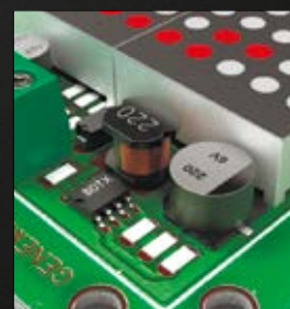
PKD230GS7 switch mode power supply
